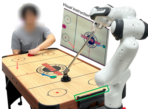
Fig. 1: A human learner learns to repel the puck into the goal region with a robot coach. The goal region is located in the middle of two ends of the table, bounded by the green box. In our Play-to-Coach system, the human learner is given visual instruction on how to repel the puck.
