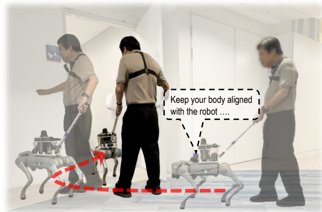
Fig. 1: CANINE. In our subject study, a robot guide dog coaches a visually impaired user to navigate through a doorway.
